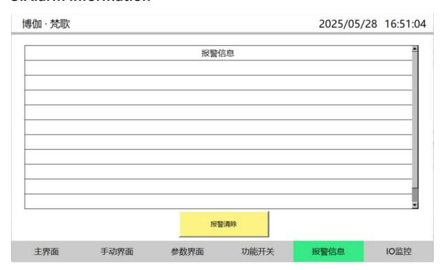
This interface will display device alarm information. When an alarm occurs, press the alarm clear button to clear some alarms
