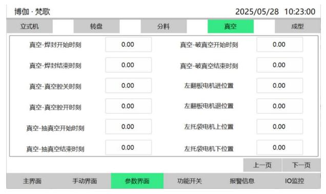
1. Vacuum welding sealing start time: This parameter is the time when the welding sealing knife in the vacuum chamber is closed. When the current time of the vacuum action cycle reaches this time, hot pressing welding sealing is carried out. The current time of the vacuum action cycle is used as the standard and cannot exceed the
